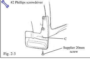
(c) Hold the part in position and drill a 2.5mm (3/32") pilot hole in location C (Fig. 2-2).
